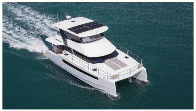
The *Cora Cat 48* takes innovation further, incorporating a bridge deck design that enhances comfort by reducing noise from wave impact. Its integrated solar array provides power for essential systems, such as air conditioning, for extended periods—an ideal solution for environmentally conscious long-range cruisers exploring remote destinations.
